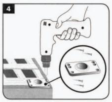
Using a power screwdriver, mount the plate to the boxspring using the supplied hardware.
