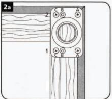
Before drilling, pick the set of screw holes you will use by measuring the width of your box-spring rail. If your rails are an actual width of 3/4" × 3 1/4", use the outside holes [C]. The side with the single set of holes [A] always faces the outside edge of the bedframe.
